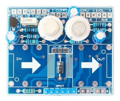
Solder the capacitors and transistors. If you have troubles reading the values, check out our <u>"Reading Part Values"</u> tutorial. Pay attention to the orientation, as well as to the polarity for electrolytic capacitors.
