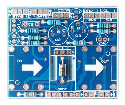
Place the resistors and diodes. If you have troubles reading the values, check out our "Reading Part Values" tutorial.
